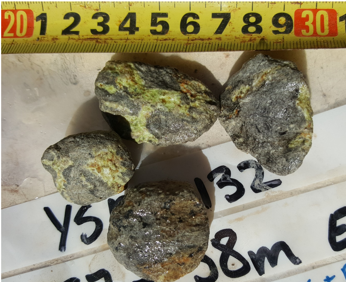
Figure 3: Bottom of hole 'core' from YSAC0132 57-58m. The rock is brecciated, with clasts of highly sulphidic silica-muscovite schist infilled by now-weathered, vuggy silica, which is interpreted as evidence of late brittle-ductile high fluid environment.
