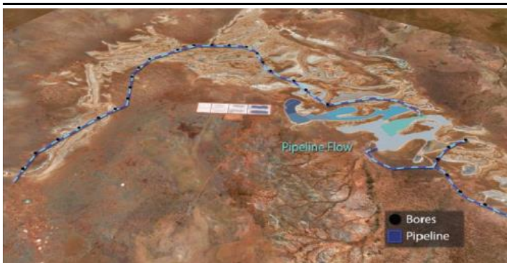
Figure 14: LWSOP borefield – 78 bores 800m spaced
