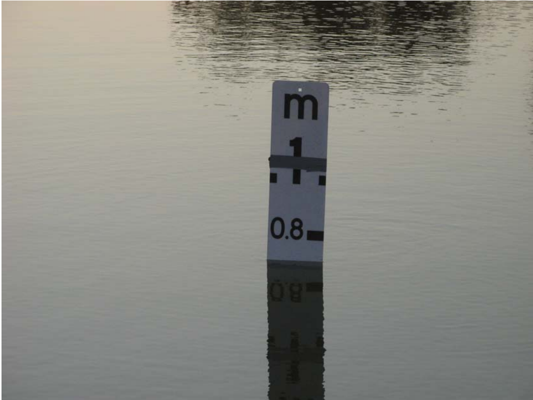
Figure 3. Fill Level in the Crystalliser Pond
