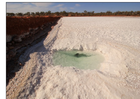
Harvest Salts precipitate as 2.2 GL/yr is evaporated from the harvest ponds, leaving 4% of original volume
