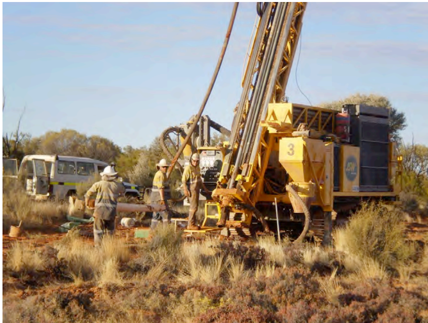
Figure 3. RC Drilling at the Axford Prospect, August, 2012.
